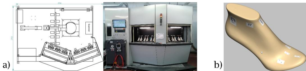
Fig. 3: a) The robot used for the marking operation, b) The shoe last virtual model with markings.
