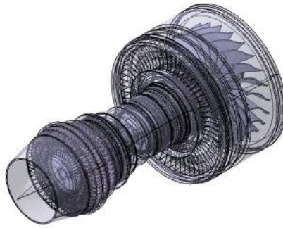
Fig. 1: Image of a turbfan engine with translucent casing showing internal bodies that are irrelevant when designing interfaces/checking clearances, etc. with the exterior casing of the assembly.
