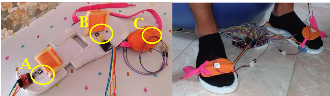
Fig. 2: On the left: slipper with vibrating motors embedded. On the right: slippers running during the simulation
