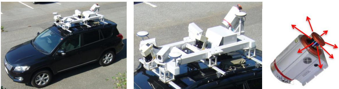
Fig. 1: Mobile mapping system: (a) Vehicle with an MMS, (b) Close-up of MMS, (c) Laser scanner.
