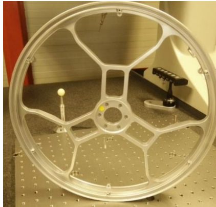
Fig. 5: Tolerance verification of the rim.
