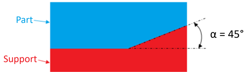
Fig. 2: Support according to angle
