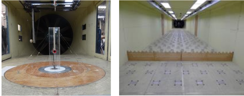
Fig. 2: (a) The physical scaled model (b) Roughness elements used in wind profile calibration.
