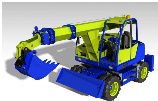
Fig. 1: Wheeled telescopic excavator based on a platform.
