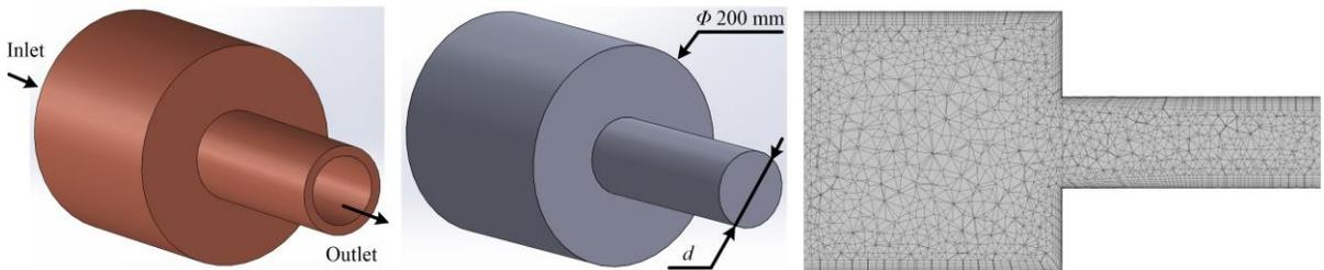
Fig. 4: Feature conversion in the analysis of the piping system: (a) Contracted pipe, (b) Fluid domain, (c) Mesh generation.
