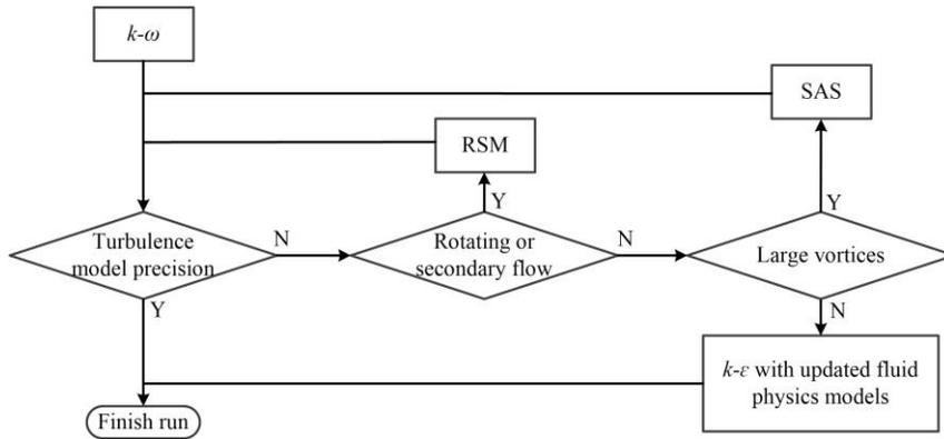
Fig. 3: Subroutine for advanced turbulence models.
