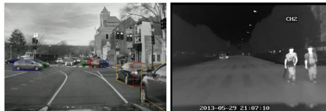
Fig. 3: Application of camera systems for object recognition: left daylight camera, right infrared camera, [6, 4].
