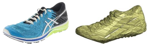
Fig. 7: Original images and triangular meshes reconstructed for example shoe.
