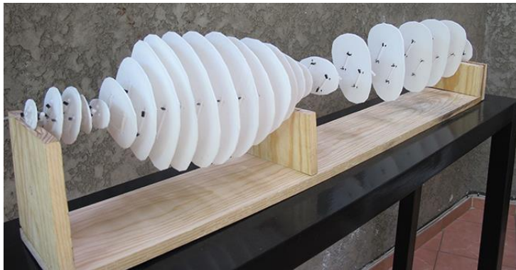
Fig. 14: Floating compression structure.
