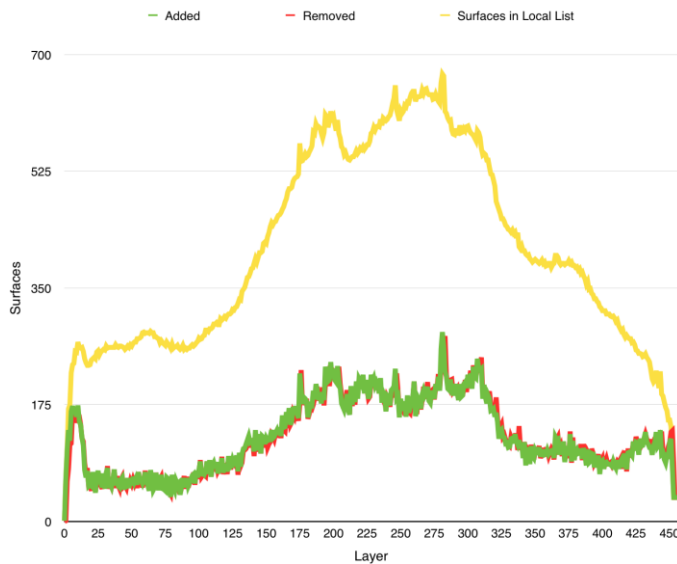
Fig. 3: Surface patch utilization of the local list: the number of added and removed surfaces are shown in green and red, respectively, while the total active surfaces are marked in yellow.
