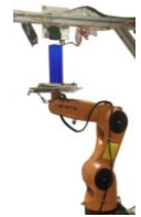
Fig. 6: Examples and results of the optimization: (a) The Y-geometry example, (b) The effect of the optimization on the number of commands for a simple and complex geometry, (c & d) The stadium geometry 3D printed on the KUKA setup proving the successful translation of G-Code to optimized KRL.
