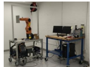
Fig. 5: From left to right: (a) Example of the scope of the post-processing workflow with the in-house developed G-code optimizer, (b) The Mendel Max 3, an off-the-shelf 3D printer controlled by G-code and (c) An in-house developed 3D Printer based on a KUKA Robotic platform used to run the converted code, controlled by KRL-code.
