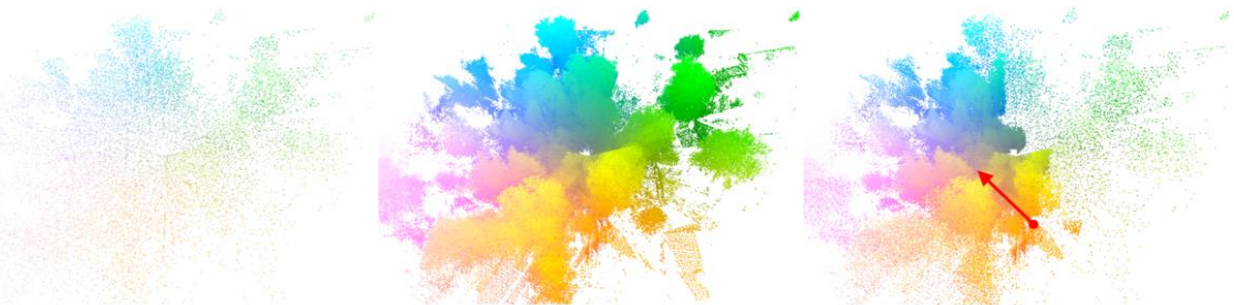
Fig. 3: Example of system on Andreas Garten dataset (45M data points). Left shows the data at points from selecting grid levels 0-7 only (48K data points). The center shows data from grid levels 0-10 (1.1M data points). The right image shows the data points gathered for a view dependent (red arrow) resolution selection (635K data points).
