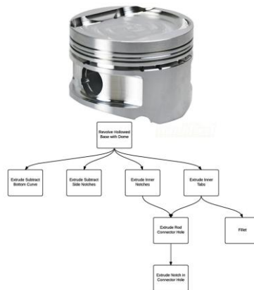
Fig. 3: Piston head and feature dependency tree.
