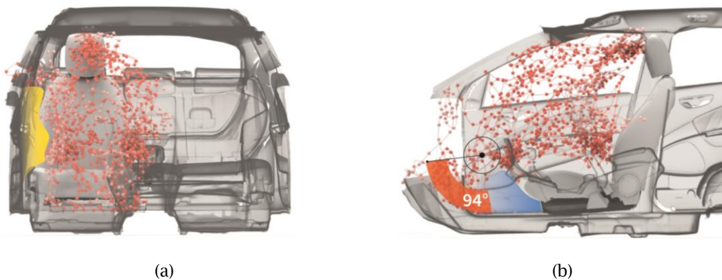
Fig. 3: Visualization of the motion data relating two actions of a single subject: (a) inclusion of a freeform geometry, (b) specific measurement of the acquired movement data.
