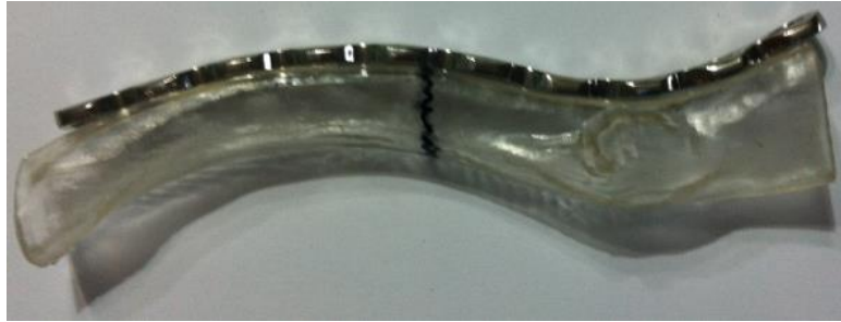
Fig. 6: Results of the bended implant fitted on the clavicle model.
