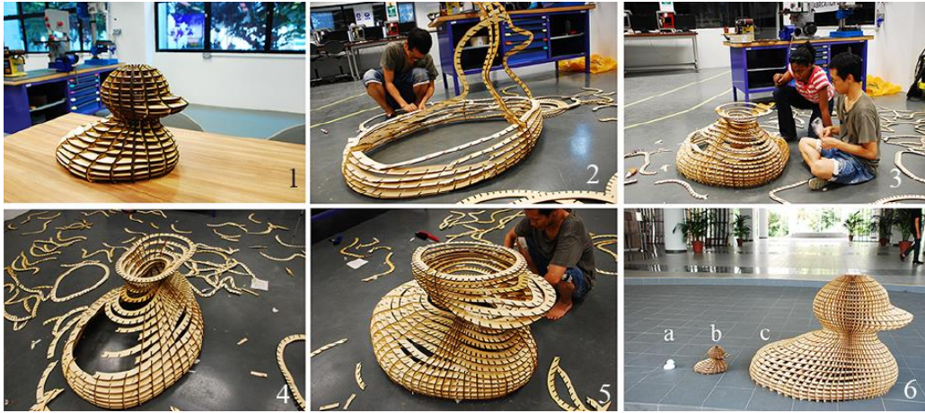
Fig. 4: (1) Middle scale model built of 20 horizontal layers. (2-6) Large-scale model: (2-3) start of assembly and base parts, (4) oscillation of joints between horizontal layers, (4-5) assembly of the last 30 layers and (6) comparison in size between original model used for scanning, middle scale and final scale build from the same scan.
