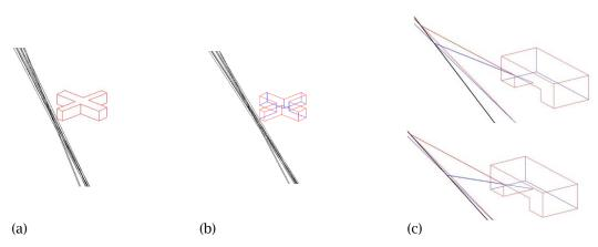
Proceedings of CAD'14, Hong Kong, June 23-26, 2014, 81-83 © 2014 CAD Solutions, LLC, <u>http://www.cad-conference.net</u> Fig. 1: (a) A given natural sketch and the cross-section generated from it, (b) the produced wireframe sketch with its hidden part geometrically reconstructed, and (c) an interactive approach is studied for sketches with ambiguous hidden part geometry.
