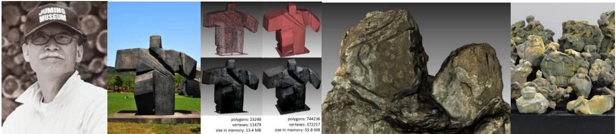
Fig. 1: The artist Ju Ming, a sculpture, the control over the resolutions of the model, 3D scanned data with image mapping and in full geometry resolution shown in high density mesh (over 7,000,000 polygons), and 3D-printed using a RP machine
