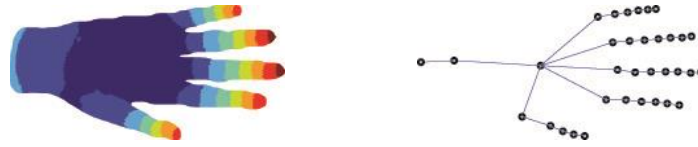
Fig. 1: Example 3D model with color-coded connected components and the corresponding graph for the same partitioning.
