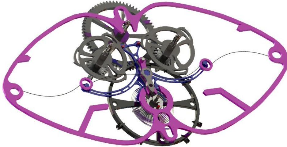
Fig. 1: The Girard-Perregaux constant force escapement.
